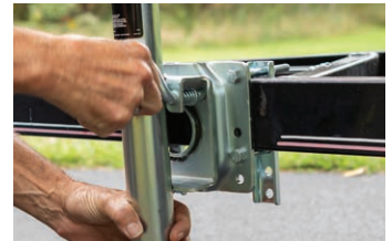
Heavy-duty pull-pin locks jack securely in place
