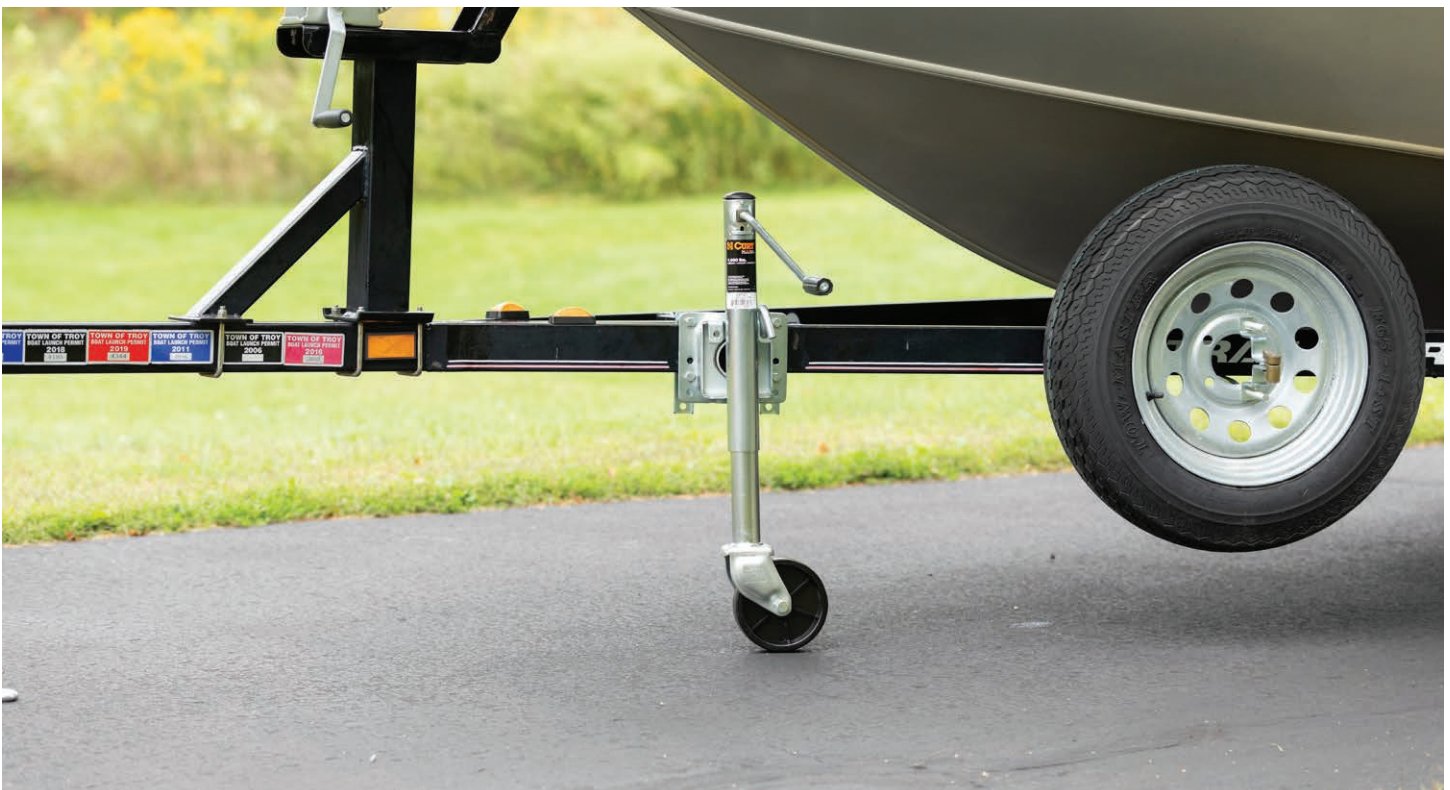
Mounting bracket can be bolted or welded to the trailer
