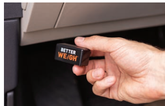
No-install, plug-and-play setup into vehicle diagnostic port (OBD-II) below the dash
